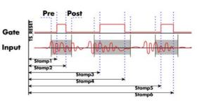
Please keep in mind that the gate signals are timestamped, not the beginning and end of the acquisition. The first sample that is available is at the time po-
