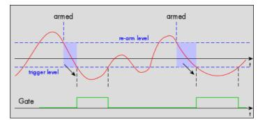
A new trigger event is only detected, if the trigger engine is armed again. The re-arm trigger modes can be used to prevent the board from triggering on wrong edges in noisy signals.
