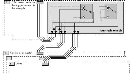
the trigger events, if all synchronized cards run with the same sampling rate. Any one of the synchronized cards can be used as a clock master and besides any card can be part of the trigger generation.
