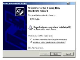
Allow Windows XP to search for the most suitable driver in a specific directory. Select the CD that was delivered with the board as installation source. The driver files are located on CD in the directory \spcm\_drv\win32 for Windows XP 32 Bit or \spcm\_drv\win64 for Windows XP 64 Bit.
