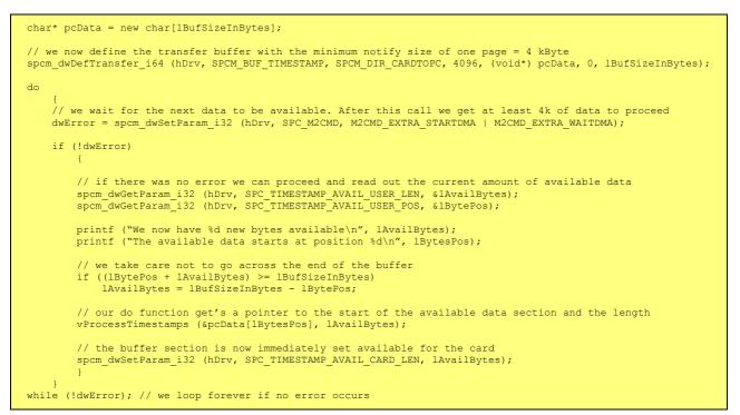
The extra FIFO has a quite small size compared to the main data buffer. As the transfer is done initiated by the hardware using busmaster DMA this is not critical as long as the application data buffers are large enough and as long as the extra transfer is started BEFORE starting the card.
