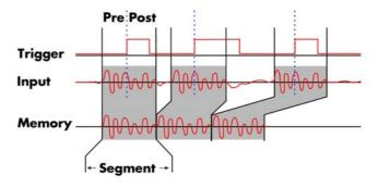
The following table shows the register for defining the structure of the segments to be recorded with each trigger event.
