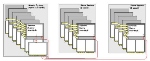
An installed master system can be extended by further systems at any time until the maximum number of systems is reached. Each of the slave systems as well as the master system can be extended by further cards until the maximum number of cards per system is reached.
