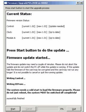
Do not abort or shut down the computer while the firmware update is in progress. After a successful update please shut down your PC completely. The re-powering is required to finally activate the new firmware version of your Spectrum card.
