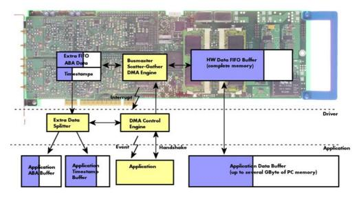
The only part that is similar for both kinds of data transfer is the handling of the DMA engine. This is similar to the main sample data transfer engine. Therefore additional information can be found in the chapter explaining the main data transfer.
