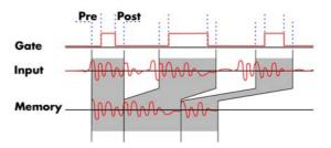
When using Gated Sampling/Replay the maximum pretrigger is limited as shown in the technical data section. When the programmed value exceeds that limit, the driver will return the error ERR\_PRETRIGGERLEN.
