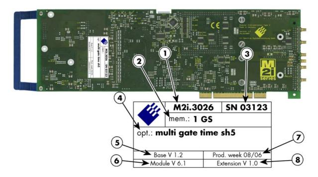
The Spectrum type plate, which consists of the following components, can be found on all of our boards. Please check whether the printed information is the same as the information on your delivery note. All this information can also be read out by software:
