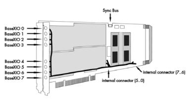
The BaseXIO MMCX connectors are mounted on-board. To gain easier access, these lines are connected to an extra bracket, that holds eight SMB male connectors. For special purposes this option can also be ordered without the extra bracket and instead with internal cables. The shown option is mounted exemplarily on a board with two modules and with the extra bracket. Of course you can also combine this option as well with a board that is equipped with only one module.
