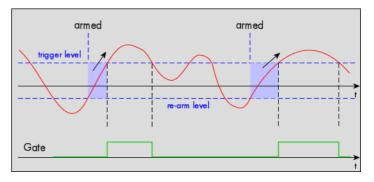
A new trigger event is only detected, if the trigger engine is armed again. The re-arm trigger modes can be used to prevent the board from triggering on wrong edges in noisy signals.
