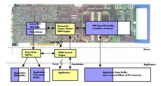
The only part that is similar for both kinds of data transfer is the handling of the DMA engine. This is similar to the main sample data transfer engine. Therefore additional information can be found in the chapter explaining the main data transfer.
