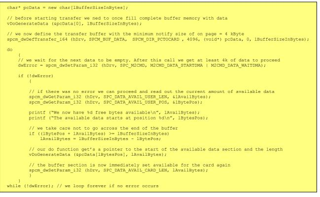
Please keep in mind that you are using a continuous buffer writing/reading that will start again at the zero position if the buffer length is reached. However the DATA\_AVAIL\_USER\_LEN register will give you the complete amount of available bytes even if one part of the free area is at the end of the buffer and the second half at the beginning of the buffer.
