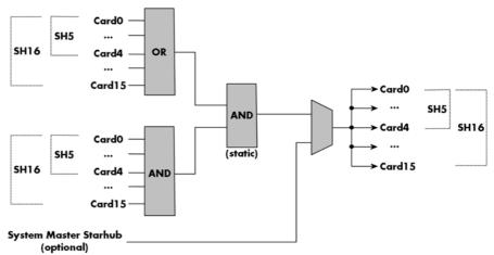
By this separation all OR masks of all synchronized cards are therefore extended to one big OR mask, while all AND masks of the synchronized cards are extended to one overall AND mask. This allows to combine the various trigger sources of all synchronized cards with AND and OR conditions and so to create highly complex trigger conditions that will certainly suit your application's needs.
