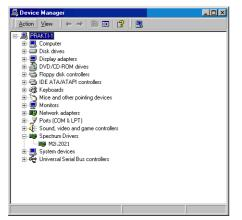
If you want to check which driver version is installed in the system this can be easily done in the device manager. Therefore please start the device manager from the control panel and show the properties of the installed driver. On the property page Windows 2000 shows the date and the version of the installed driver.
