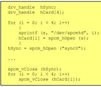
When opening the Star-Hub the cable interconnection is checked. The Star-Hub may return an error if it sees internal cabling problems or if the connection between Star-Hub and the card that holds the Star-Hub is broken. It can't identify broken connections between Star-Hub and other cards as it doesn't know that there has to be a connection.
