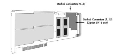
clock and trigger signals. Each board is connected with a small cable of the same length, even the master board. That minimizes the clock skew between the different cards. The figure shows the piggy-back module mounted on the base board schematically without any cables to achieve a better visibility. It also shows the locations of the available connectors for the two different versions of the star-hub option.
