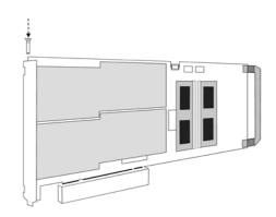
Installing the M2i.xxxx PCI/PCI-X card in a 64 bit PCI/PCI-X slot
