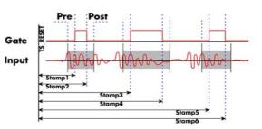
Please keep in mind that the gate signals are timestamped, not the beginning and end of the acquisition. The first sample that is available is at the time po-
